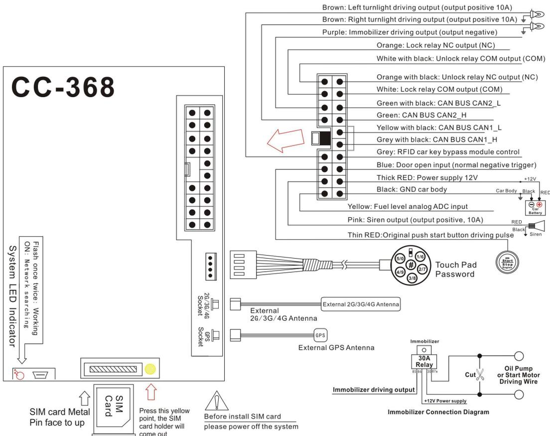
The immobilizer output can be used to control the car starting motor or oil pump motor line or ON line, etc. Please note a 30A relay need to connect to the immobilizer wire to control the engine off. The immobilizer output is an open-circuit negative output (load current 500mA), which can only drive the relay and cannot be directly connected to the circuit of the car. The relay is connected as shown below:
