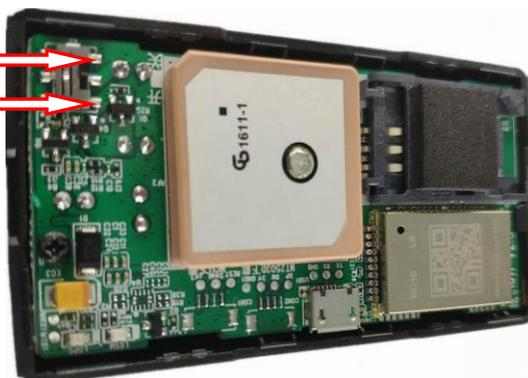
After power on the tracker will begin to work, the LED light will flash, first close the shell, put the tracker outside, after 5-10 minutes, see if the position of the tracker is updated, if the position has been updated, it means the tracker is normal.
