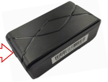
Slide the top cover of the SIM card holder to OPEN direction to release SIM card. push & slide the cover to the LOCK direction to lock the SIM card.
