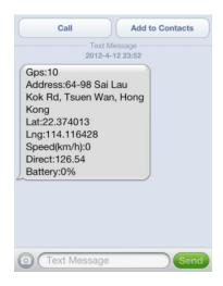
If the tracker can not get the location text description, the tracker will reply the location with Google map link SMS to user, please refer the following 3. And If no GPS signal in that place the tracker will locate by LBS (Cell ID GSM network base station), and reply the LBS location with Google map link. please refer the following 4.
